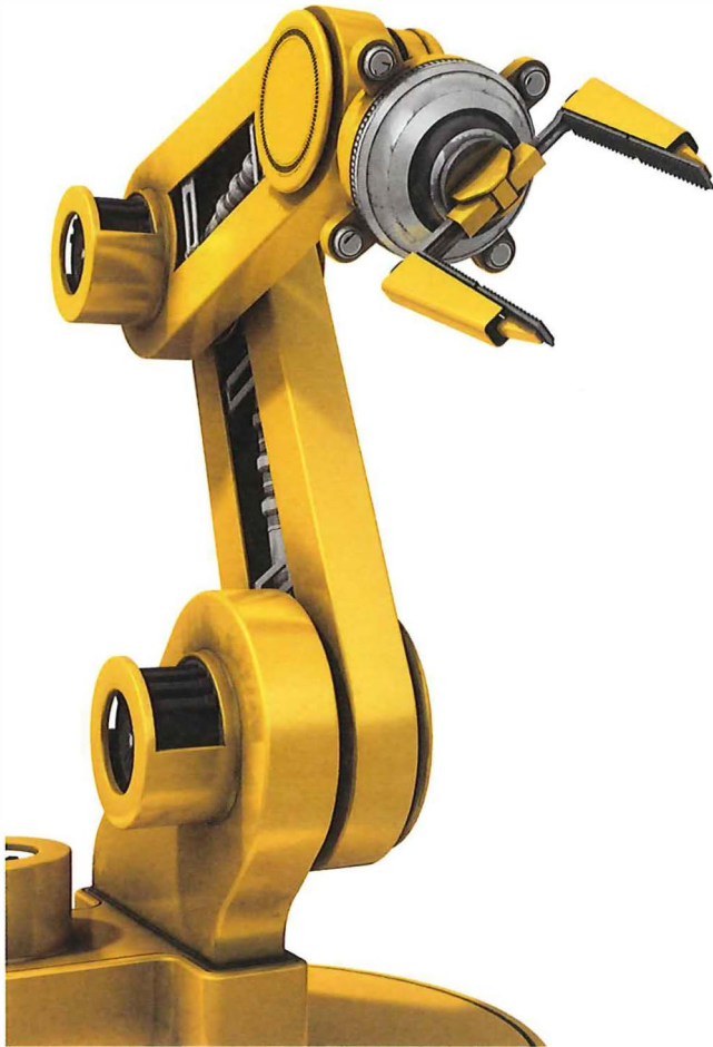
Figure 7.08 Actuators are used to produce the movement of a robot arm
