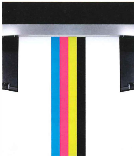
Figure 7.03 Printers use a mixture of cyan, magenta, yellow and key (black) to create different colours
